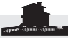
The land should have a very slight incline which would allow surface water to drain towards the street.
