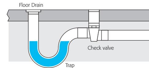
In the event of heavy precipitations, especially when there is a lot of surface water, your valves may shut off in order to play their protective role. Be careful! When you flush the toilet and your valves have already shut off to control backflow, they will also block all other water flow. You run the risk of flooding yourself!
